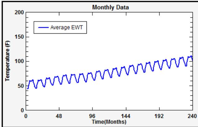
**Figure 4** This graph shows the expected GHX temperatures that can be expected based on the energy load profile in figure 3(b). All of the thermal energy dissipated through the radiator of the diesel generator is rejected to the GHX. Over a 20 year period the GHX temperature can be expected to climb to over 110°F (43°C). The GHX field in this model is based on 500 boreholes to a depth of 400' (122 m) for a total of 200,000' (60,957 m) of drilling.
