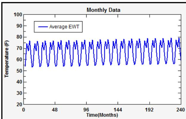
**Figure 6** After construction of the GHX is complete and most of the buildings are connected to the system, the amount of energy rejected to the GHX is controlled to maintain the optimum operating temperature.
