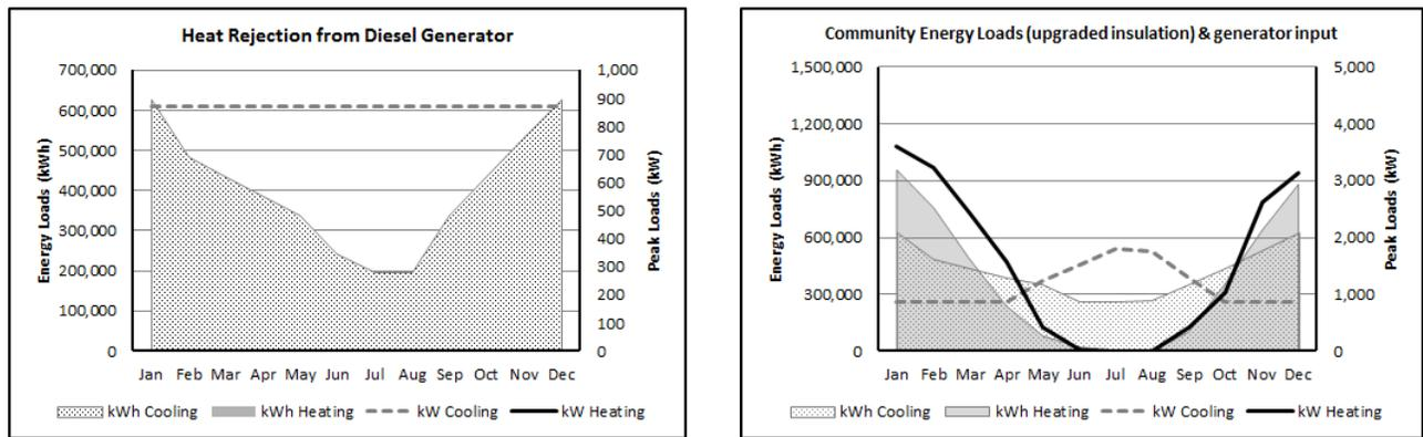
a) (b) **Figure 3** (a) This graph illustrates the total amount of waste energy that can be rejected to the GHX from the diesel generator. (b) This graph illustrates the total community building heating energy load profile with the waste heat rejected from the diesel generator overlaid on it. The load profile used in this graph assumes the insulation and construction of the residential buildings have been upgraded to reduce the heating loads.
